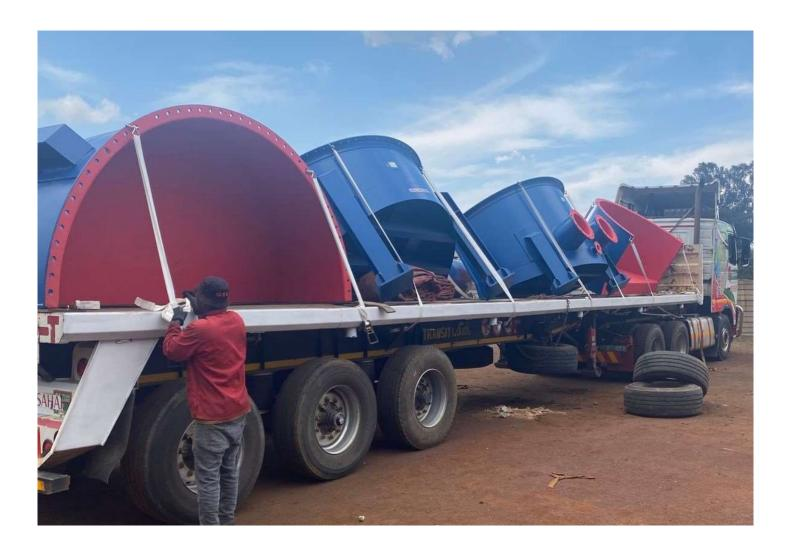
Transport jigs were designed and built to brace the components and reduce vibration during the trip.
