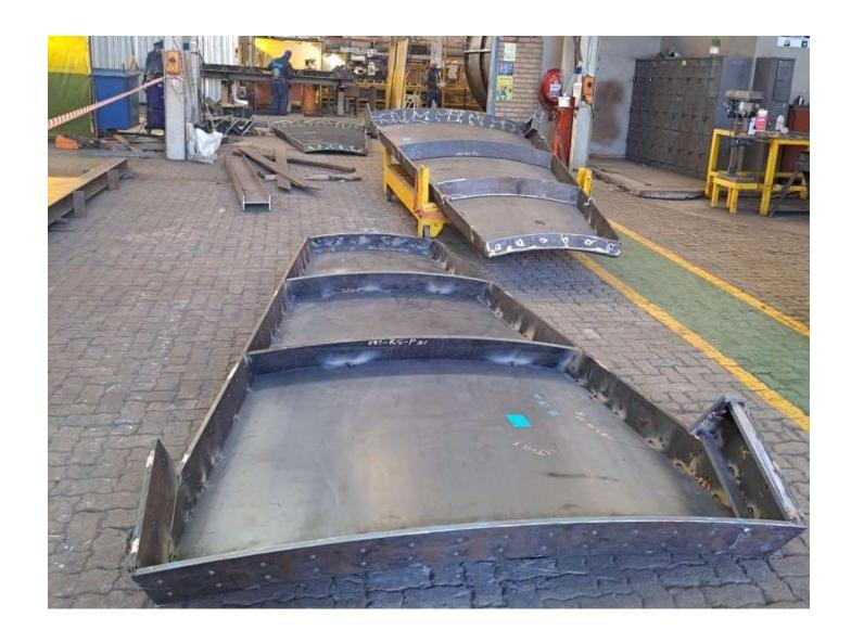
The first Reactor was trial assembled to prove that the jigs and manufacturing was correct.
