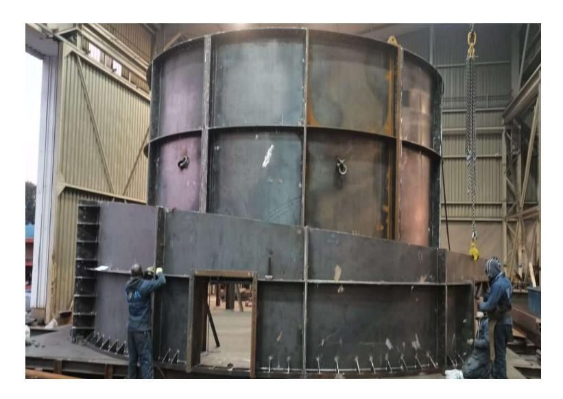
Six Reactor tanks each 9.9m in diameter and 11.6m high were fabricated and supplied to the project
