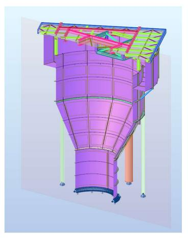
The splices or connections between each piece of the structure also form the stiffeners required for out of plane forces due to the geometry (such as at the transition points between cylindrical and conical forms) and externally applied loads (such as the supported platform, wind and equipment loads).
