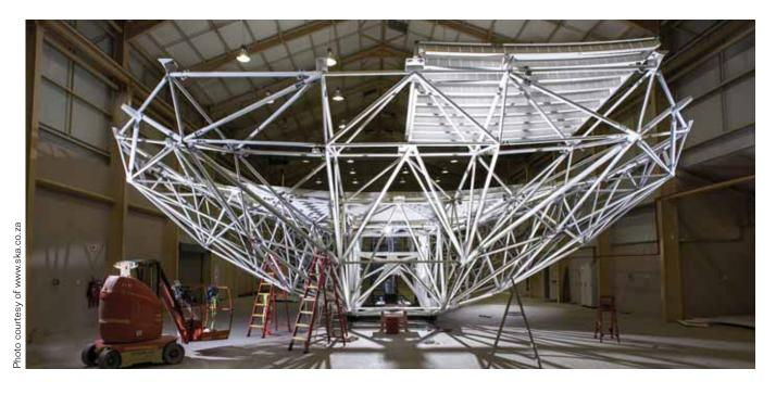
Prevention of distortion from welding to the yoke is just one of the many challenges faced by the fabrication team. The judges thought this was excellent use of plated steelwork highlighting the versatility of the fabricator's repertoire. The steelwork contractor is usually associated with tower steelwork.
